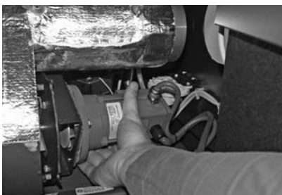
Fig. 154 Removing wing nuts, removing the blower unit
