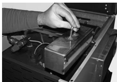
Fig. 144 Removing the jet protection plate
