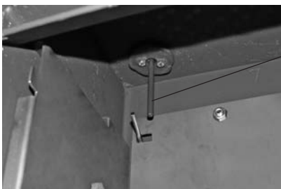
Fig. 127 Cleaning the temperature sensor (with cleaning brush)
