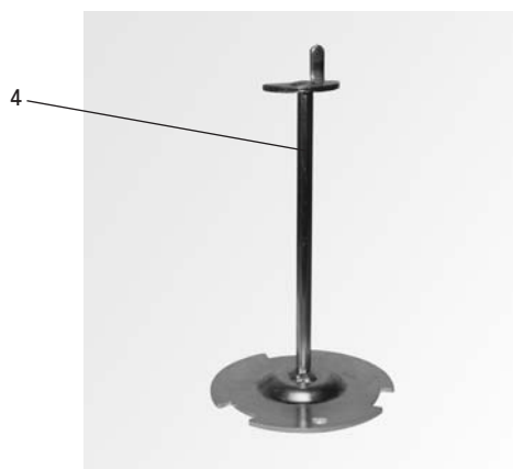
Fig. 121 Cone removal tool and grate removal tool
